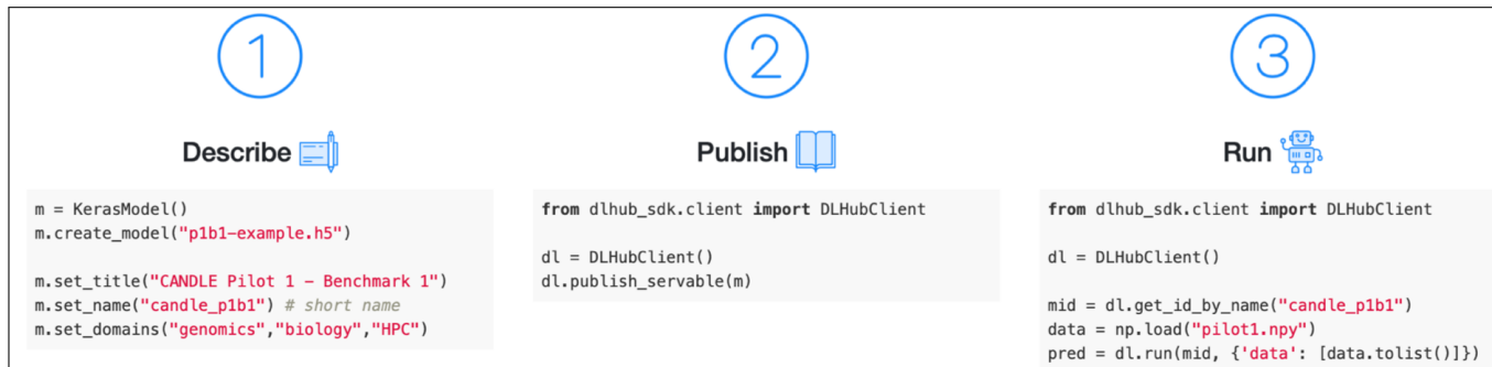
Figure 1: Illustrative uses of DLHub Python APIs, here used to (1) assemble a description of a model, with relevant metadata; (2) publish the new model to DLHub; and (3) invoke the published model.
